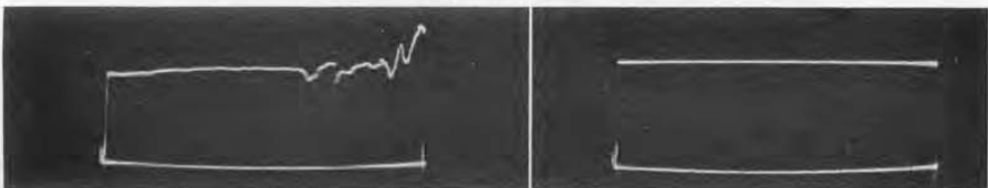
Figure 11. Output amplitude characteristic as a function of frequency for the Type 1209-B Unit Oscillator (250-920 Mc), unregulated (left), and (right) when operated from the Amplitude-Regulating Power Supply.
