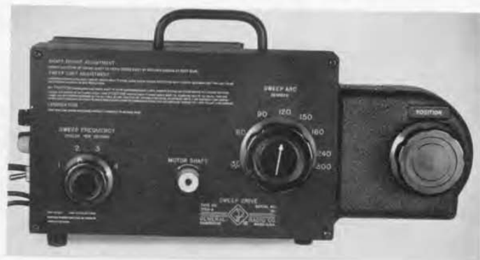
Figure 2. Front panel view of the Type 1750-A Sweep Drive, showing the SWEEP FREQUENCY, SWEEP ARC, and POSITION controls.
