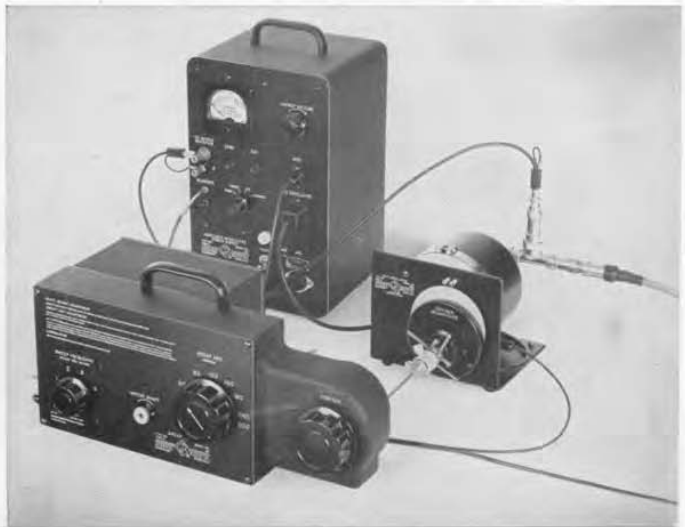
Figure 1. View of the new General Radio Sweep Drive and Amplitude-Regulating Power Supply set up to sweep a Type 1209-B Unit Oscillator.
